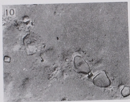
6. Automorphic "cubic" inclusion, \times 12\ 200 . 7. Automorphic "cubic", two-phase inclusion, \times 600 . 8. Automorphic inclusion with three-fold symmetry, \times 12\ 200 . 9. Xenomorphic inclusion, \times 12\ 200 . 10. Xenomorphic inclusions on a healed fracture, \times 12\ 200 . Photos. 6, 8, 9, 10. Images from the electron microscope, replicas
